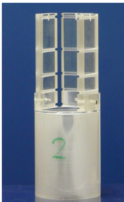
Fig. 3.8: The stack holder used for placing the activated stack in front of the Si-Li detector 2. Of the five possible positions only the lower has been used. See the text for details.
