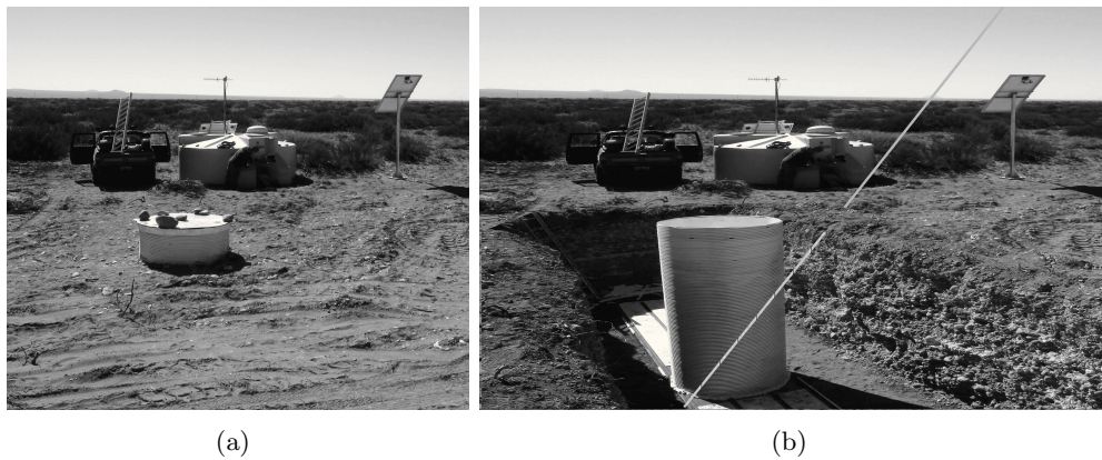
Figure 4.11: 4.11(a): Surface infill SD station with its associated muon counter already buried. Once instrumented, the access pipe is filled with bags containing soil from the installation site. 4.11(b): Photograph to depict the detector concept: any impinging muon with energy \geq 1 \text{ GeV} propagates in the soil and is capable of reaching the buried scintillator.
