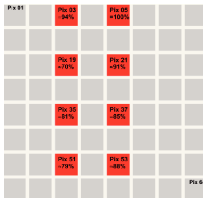
Figure 4.19: PMT relative pixel uniformity: non-uniformity can be as high as 30% in the center of the PMT pixel grid.
