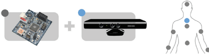
Fig 97. Hardware modification for combined SLAM and MOCAP approach. The iNEMO-based solution for inertial movement reconstruction has been linked to a Microsoft Kinect-based solution for environment reconstruction.
