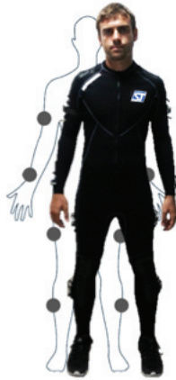
Fig 93. MOCAP interesting points in human body. In its simplest implementation it counts 10 sensors: two per each limb plus two through the spine. Additional sensors could be mounted on wrist, ankles and head.
