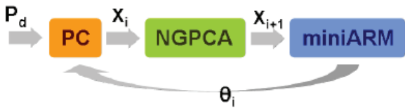
Fig 64. Algorithm block diagram for sequence learning with Neural Gas with local Principal Component Analysis (NGPCA). The Pattern Constructor block (PC) performs control modifying the input pattern with the oset P_d . The miniARM block is the serial redundant manipulator (controlled in the operating space).
