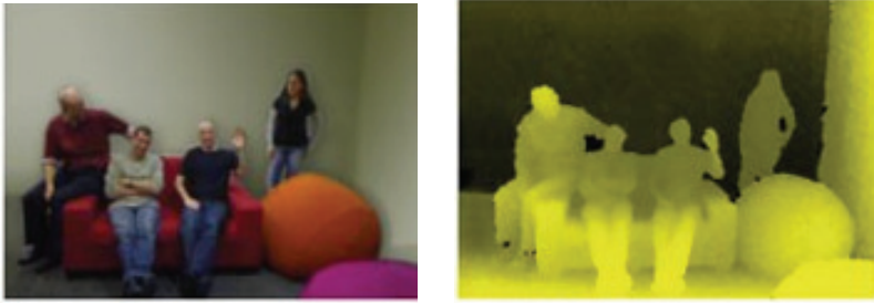
Fig 98. RGB-D camera images. The colour information is depicted on the left (RGB) while the depth information is on the right (monochrome) (pictures from prime sense website).
