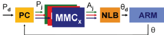
Fig 80. Control scheme for each arm for a given absolute reference input pattern, P_d . PC is the Pattern Constructor, MMC_x , MMC_y and MMC_z are the three-dimensional linear computational networks. NLB is the Non-Linear Block and ARM is the manipulator itself (simulator or real robot). P_j are the MMC input pattern while A_j are the outputs. \theta_d are the desired angular values and \theta are the read joints values.
