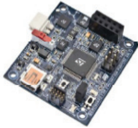
Fig 6. iNEMO™ evaluation board from STMicroelectronics: 10 DoF demonstration board based on accelerometer, gyroscope and magnetometer. It integrates a common quaternion based Kalman filter.
