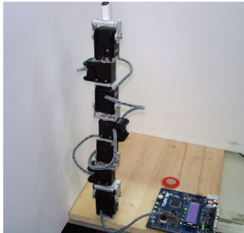
Fig 27. Experimental setup with the real robot (7-DoF manipulator) and the 32 bit microcontroller board.
