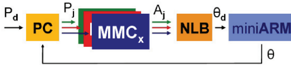
Fig 22. Algorithm block diagram for a given absolute reference input pattern, P_d . PC is the Pattern Constructor, MMC_x , MMC_y and MMC_z are the three-dimensional linear computational networks. NLB is the Non-Linear Block and miniARM is the manipulator itself (simulator or real robot). P_j are the MMC input pattern while A_j are the outputs. d are the desired angular values and \theta are the read joints values.
