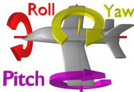
Figure 16. Graphical explanation of the angles of roll (rotation around the X axis), pitch (rotation about the Y axis) and yaw (rotation around the Z axis).
