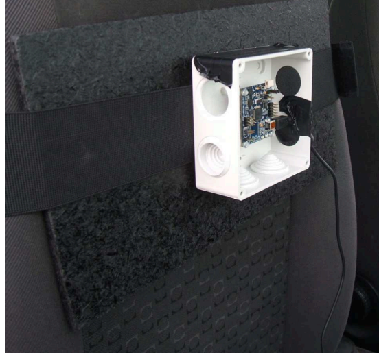
Figure 86. Fixing the inertial platform.
