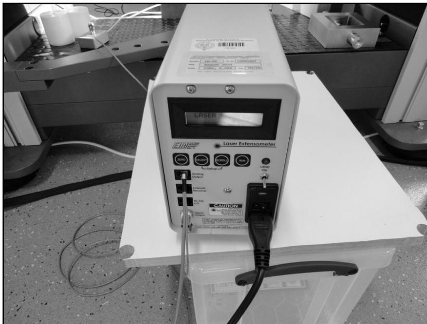
**Figura H.12 - Estensometro Laser Electronic Instrument Research LE - 05**
