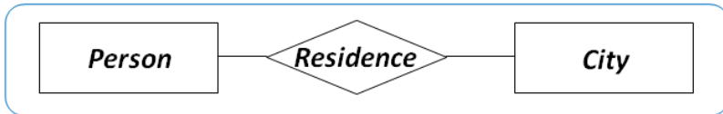
Figure 57 – Example of the graphical representation of relation between two entities: The person is related to the city with his residence
