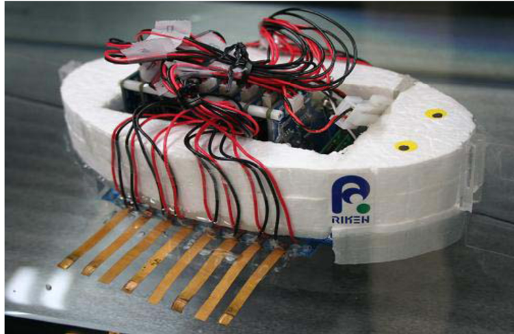
Figure 1.11: Aquatic robot with 8 IPMC strips for each fin
