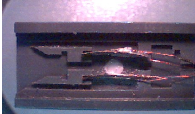
Figure 1.13: A photograph of the fabricated double-diaphragmpump. The size of the IPMC is 1 mm width \times 5 mm length \times 0.2 mm thickness [2].
