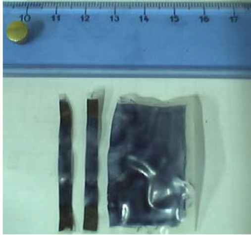
Figure 1.16: Samples prepared by drop-casting technique.
