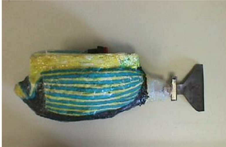
Figure 1.12: Robotic fish equipped with a single IPMC tail fin
