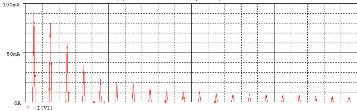
Figure 4.7: Fourier analysis of the line current ( f_{\text{cutoff}} = 1/10 f_{\text{sw}} ).
