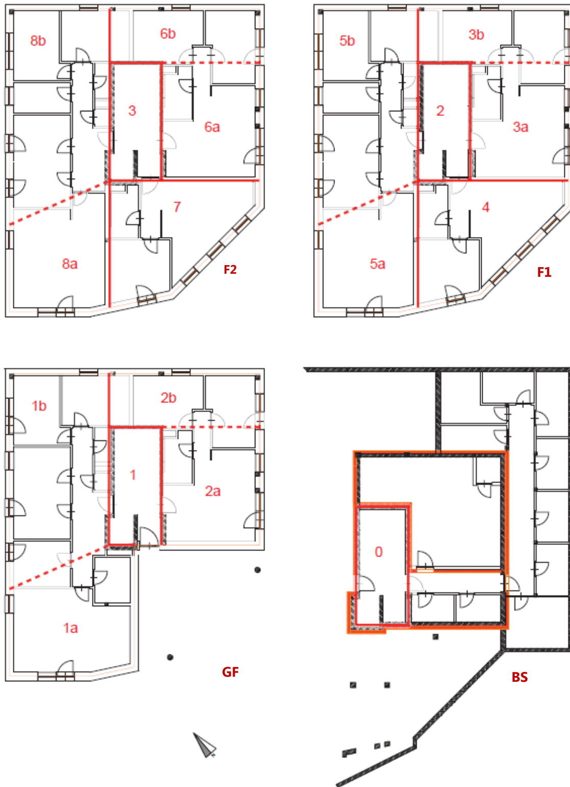
Fig. 2.5 Zone partitioning of basement (BS), ground floor (GF), first (F1) and second (F2) floor
