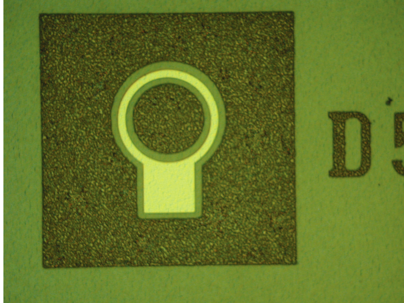
Fig. 5.22: Picture of a fabricated round HEMT on AlGaN/GaN heterostructures on Al 2 O 3 substrates.
