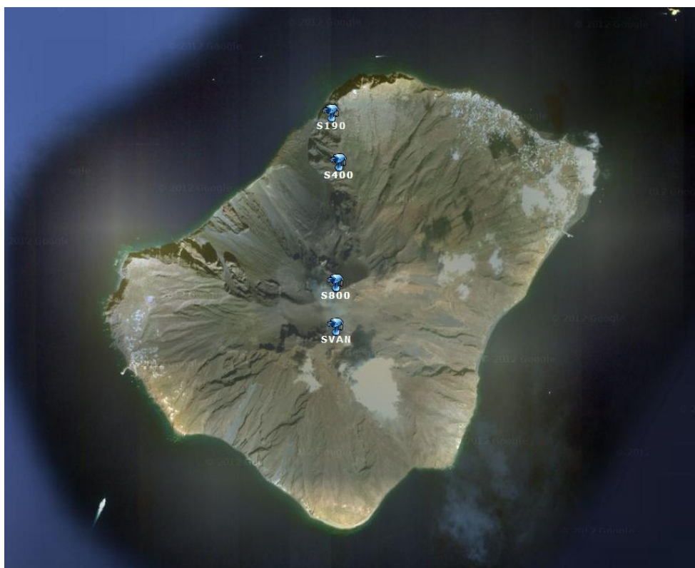
Figure 40 – Map of thermal cameras monitoring the activity of Stromboli Volcano in Stromboli Island (Aeolian Islands, Italy). There are 3 thermal cameras, located at Pizzo (S400 and S800) and Vancori (SVAN)
