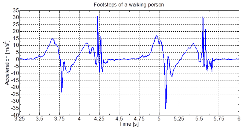
Fig. 3.2 – Time series of the acceleration coming from the footsteps of a walking person, measured through an accelerometer placed near the heel.
