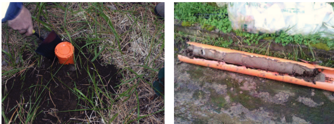
Figure 3.10 - Closed PVC tube introduced inside the borehole at Vena (left picture). Soil-filled PVC tube located in the vicinity of SVF (right picture).
