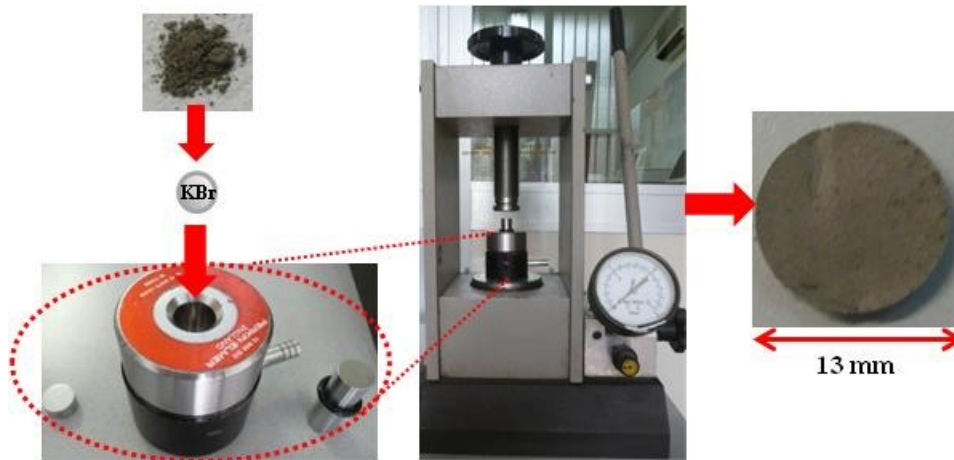
Fig. 2.15 – The cylindrical sample holder and the press used to prepare sample's pellets.
