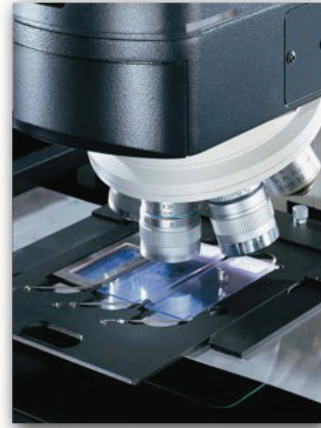
Figure 7 – The Leica micro-dissection microscope used to count and analyze the stomata on the adaxial and abaxial Miscanthus leaves grown and measured at different growth temperature.
