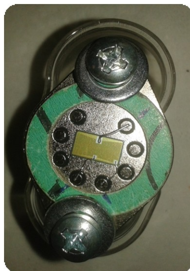
Figure 85: Nude MOSFET, prepared to coating.
