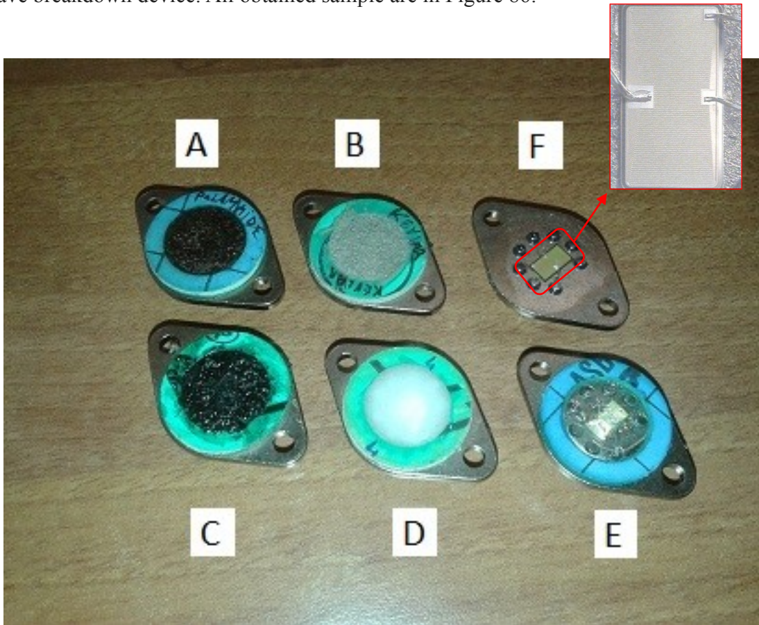
Figure 86: Several composite deposited on device; KAP.33 (A), KEV.33 (B); GO.33 (C) SIL.33 (D), Resine (E), bare die (F).
