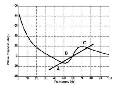
Fig. 51: Waveforms of islanding detection with slip mode frequency shift method-
