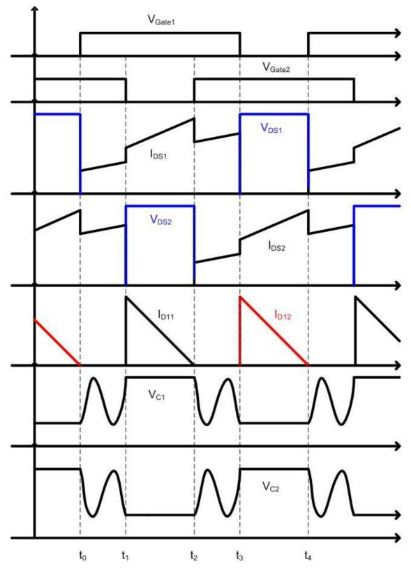
Fig. 29: Wave forms of the proposed converter.
