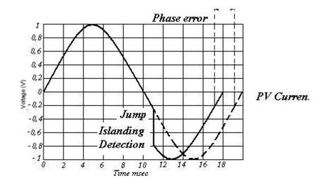
Fig. 50: Waveforms of islanding detection with voltage phase jump detection method
