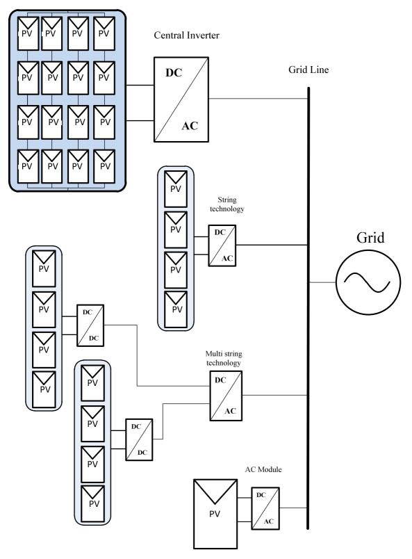
Fig. 6: PV topology; central inverter, string converter, multi string converter and ACModule.
