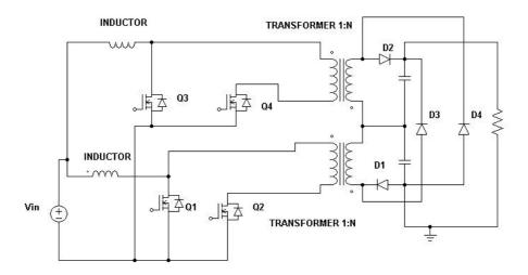
Fig. 10: L-type Half-Bridge Interleaved Isolated Boost converter.
