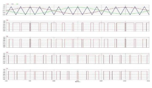
Fig. 62: Unipolar PWM modulation
