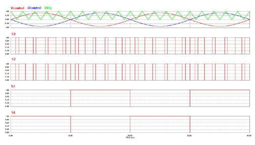
Fig.64: Hybrid PWM modulation
