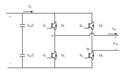
Fig. 59: Full Bridge inverter schematic
