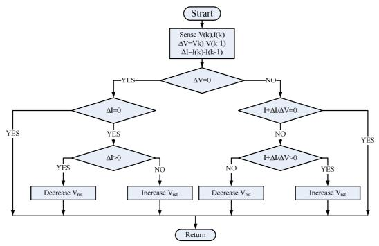
Fig. 43 Flow chart of InC MPPT algorithm.
