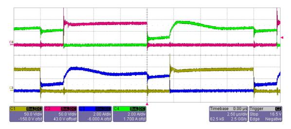
Fig. 18 Experimental results. Ch1 (Yellow): S1 Drain-Suorce Voltage; Ch2 (Red): S2 Drain-Suorce Voltage; Ch3 (Blue): S1 drain-source current; Ch4 (Green): S2 source current.
