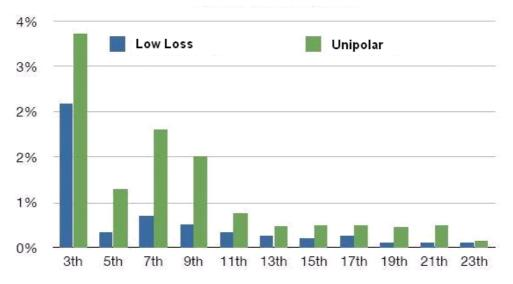
Fig. 66: Harmonic distortion comparison between mixed frequency PWM technic and Unipolar technic
