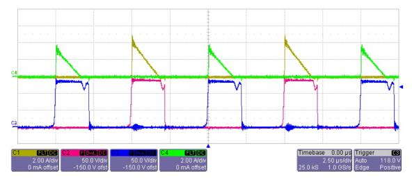
Fig. 35: Experimental results using Fast-Diode: Ch1 (Yellow) Diode current (D<sub>21</sub>). Ch2 (Red) S<sub>2</sub> drain-source voltage; Ch3 (Blue) S<sub>1</sub> drain-source voltage; Ch4 (Green) Diode current (D<sub>11</sub>).
