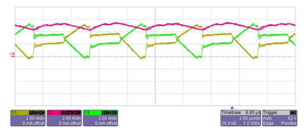
Fig. 31: Experimental results. Ch1 (Yellow): S2 source current; Ch2 (Red): L boost current; Ch4 (Green): S1 source current.
