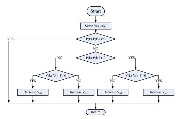
Fig. 42: Flow chart of P&O MPPT algorithm
