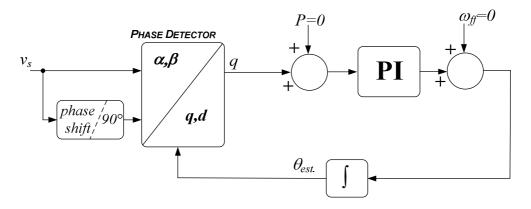
Fig. 72: Orthogonal system generation based PLL scheme (O PLL).
