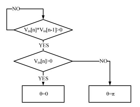
Fig. 45: Flowchart of zero-cross-detection method
