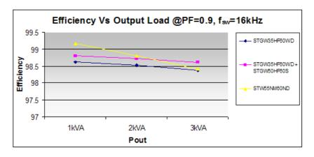
Fig. 86: Efficiency as a function of output load at fsw=16kHz, PF=0.9
