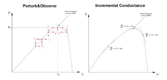
Fig. 41: Operation of two MPPT algorithms.
