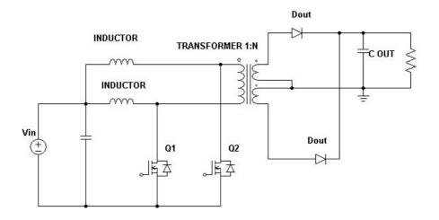
Fig. 7 Boost-Interleaved Converter with HF Transformer.
