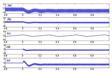
Fig 76: Voltage dips test.(a) P\_PLL, (b) E\_PLL, (c) X\_PLL, (d) O\_PLL, (e) I\_PLL.x-axis: Time [s], y-axis: errors [degrees].
