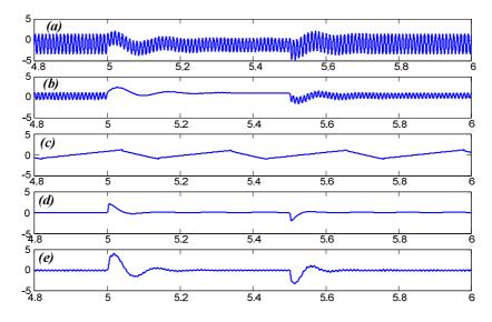
Fig. 75: Phase error during a voltage sag test.(a) P\_PLL, (b) E\_PLL, (c) X\_PLL, (d) O\_PLL, (e) I\_PLL.x-axis: Time [s], y-axis: errors [degrees].
