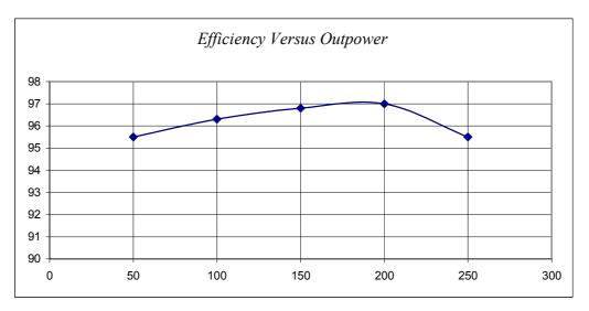
Fig. 23: Effciency versus Power for 3 stage and 36 V input voltage and 400 V output voltage
