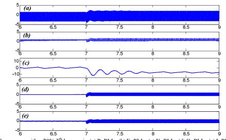
Fig. 74: Phase error with a 20% 3<sup>th</sup> harmonic.(*a*) P\_PLL, (*b*) E\_PLL, (*c*) X\_PLL, (*d*) O\_PLL, (*e*) I\_PLL*x*-axis: Time [s], y-axis: errors [degrees].
