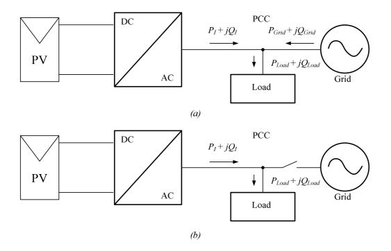
Fig. 53: Power flows in normal (a) and islanding (b) conditions
