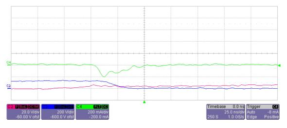
Fig. 37: Experimental results using SiC-Diode: Ch2 (Red) S<sub>1</sub> gate-source voltage; Ch3 (Blue) S<sub>1</sub> drain-source voltage; Ch4 (Green) Diode current (D<sub>11</sub>).
