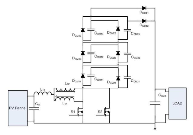
Fig. 26: Scheme of Multi-Cell converter
