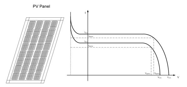
Fig. 4 PV-Cell and V-I characteristic
