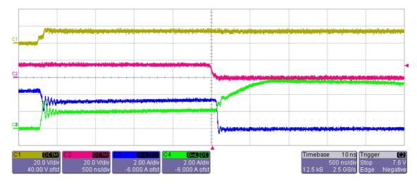
Fig. 21: Experimental results. Ch1 (Yellow): S2 gate-voltage; Ch2 (Red): S1 gate-source voltage; Ch3 (Blue): S1 drain-source current; Ch4 (Green): S2 source current.
