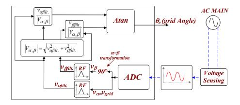
Fig. 46: PLL Block diagram of technique based on Stationary Reference Frame Transformation
