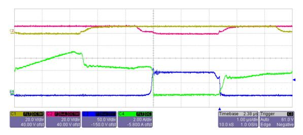
Fig. 34: Experimental results. Ch1 (Yellow): S2 gate-source voltage; Ch2 (Red): S1 gate-source voltage; Ch3 (Blue): S1 drain-source voltage; Ch4 (Green): S1 source current.
