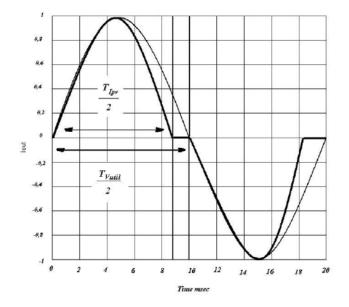
Fig. 52: Waveforms of islanding detection with active frequency drift method
