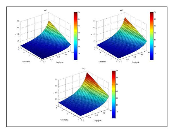
Fig. 30.:Voltage gain of the proposed converter as a function of duty cycle and turn ratio obtained with 1 (a), 2 (b) and 3 (c) Multi-cell stages.
