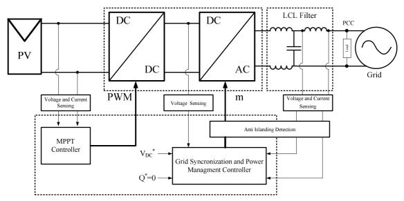
Fig. 55: Control scheme of a grid-connected converter
