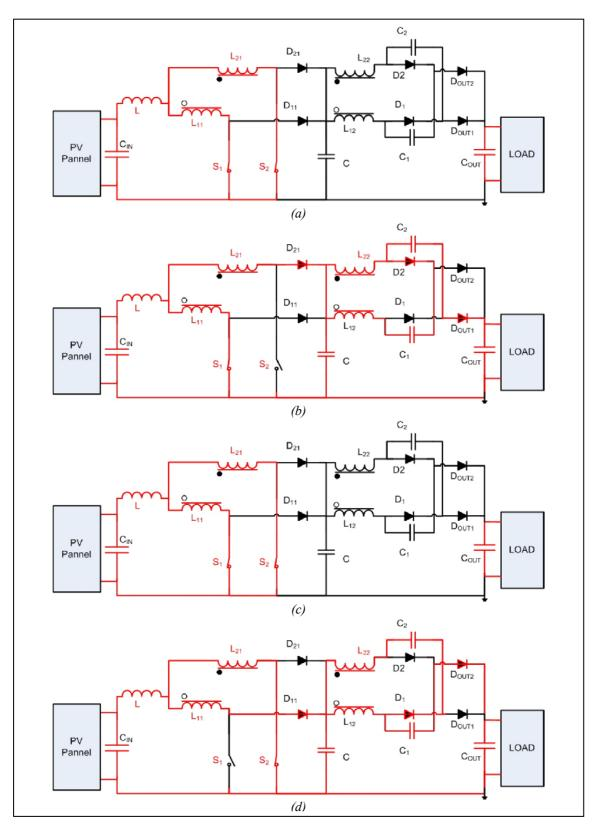
Fig. 28: Operation analysis of the proposed converter.
