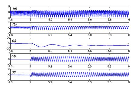
Fig. 79: Offset Rejection.(a) P\_PLL, (b) E\_PLL, (c) X\_PLL, (d) O\_PLL, (e) I\_PLL. x-axis: Time [s], y-axis: errors [degrees]
