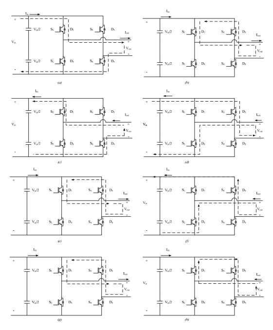
Fig. 65: State of commutation for Hybrid PWM modulation
