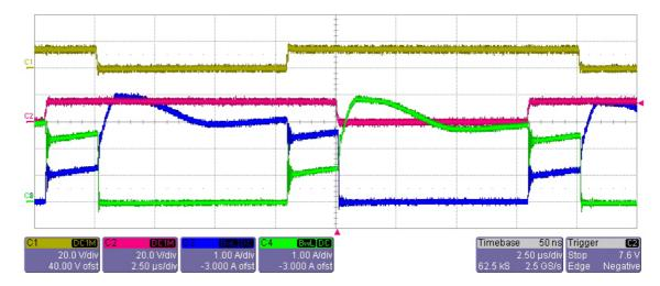
Fig. 20: Experimental results. Ch1 (Yellow): S2 gate-voltage; Ch2 (Red): S1 gate-source voltage; Ch3 (Blue): S1 drain-source current; Ch4 (Green): S2 source current.
