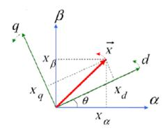
Fig. 56: Vector representation of stationary ( $\alpha\beta$ ) and synchronous (dq) rotating frame
