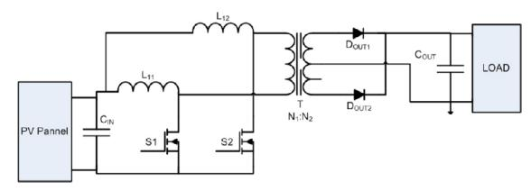
Fig. 24: Scheme of interleaved boost converter with HF transformer
