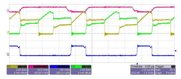
Fig. 32: Experimental results. Ch1 (Yellow): S2 source current; Ch2 (Red): S1 gate-source voltage; Ch3 (Blue): S1 drainsource voltage; Ch4 (Green): S1 source current.
