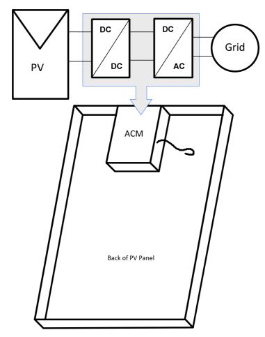
Fig. 5: Basic topology of an ACModule
