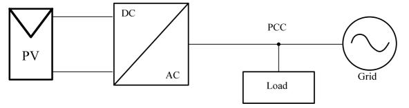
Fig. 49: Block scheme of PV generator connection with the grid
