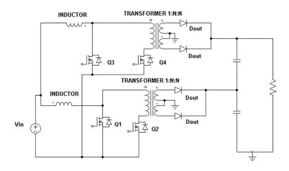
Fig. 8 Dual Boost-Interleaved converter with HF Transformers
