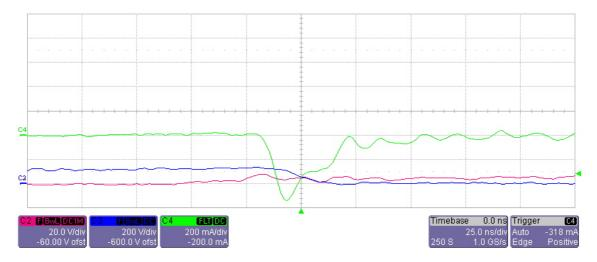
Fig. 36: Experimental results using Fast-Diode: Ch2 (Red) S<sub>1</sub> gate-source voltage; Ch3 (Blue) S<sub>1</sub> drain-source voltage; Ch4 (Green) Diode current (D<sub>11</sub>).
