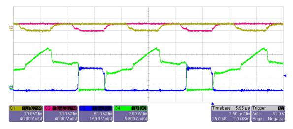
Fig. 33: Experimental results. Ch1 (Yellow): S2 gate-source voltage; Ch2 (Red): S1 gate-source voltage; Ch3 (Blue): S1 drain-source voltage; Ch4 (Green): S1 source current.
