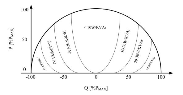
**Fig. 82:** Relative additional losses [W/kVAr] of reactive power supply Q [%Pmax] of an inverter with 96% maximal efficiency generating active power P [%Pmax]
