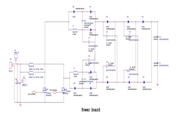
Fig. 14: PSpice Schematic ot the Multi-Cell Power Bord
