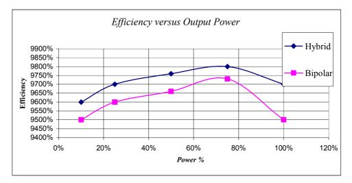
Fig. 68:: Inverter efficiency of the PV converter
