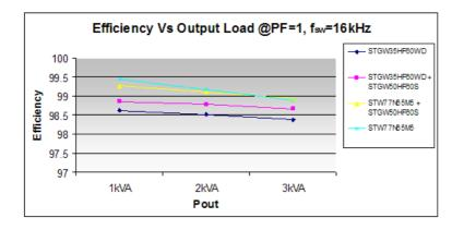
Fig. 85: Efficiency as a function of output load at fsw=16kHz, PF=1
