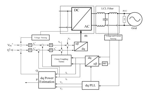
Fig. 57: Scheme of the power management control
