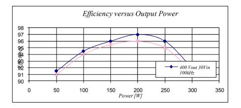
Fig. 40: Efficiency at 400V output. Input 30V (blue), 36V (red).
