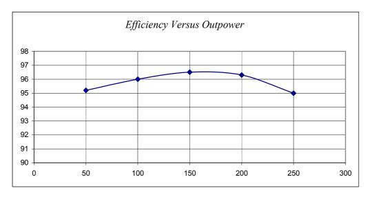
Fig. 22: Effciency versus Power for 3 stage and 24 V input voltage and 200 V output voltage
