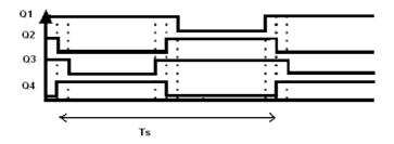
Fig. 9. PWM signal for the dual boost-interleaved converter with HF Transformers
