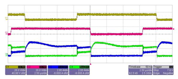
Fig. 19: Experimental results. Ch1 (Yellow): S2 gate-voltage; Ch2 (Red): S1 gate-source voltage; Ch3 (Blue): S1 drain-source current; Ch4 (Green): S2 source current.
