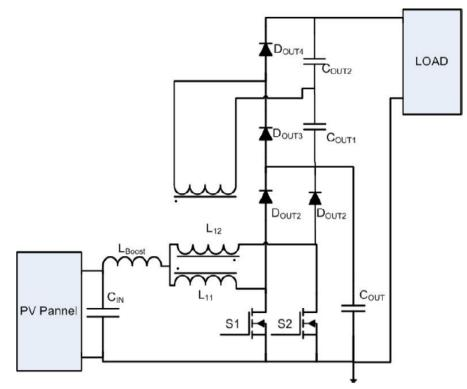
Fig. 25: Scheme of Multi-Stage converter.
