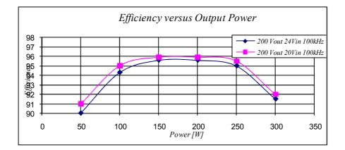
Fig. 39: Efficiency at 200V output. Input 24V (red), 20V (blue).
