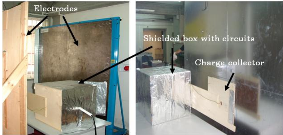
FIGURE 4-21 Experimental setup. The two large electrodes (2 m x 2 m each) and the guard chamber are shown in (a); the charge collector is visible in (b).
