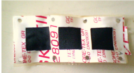
Fig. 3.12: Gore-Tex ® expanded PTFE sealing for the three cell planar stack. There are visible the three electrodes (in black), meanwhile the sealing is the white frame around the electrodes.
