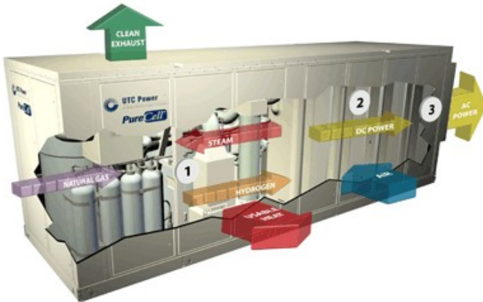
Fig. 1.8: PureCell stationary fuel cell power system, by UTC Fuel Cells. The system has been installed in several locations worldwide. It can provide electric power as well as heat with very low emissions and high performances. Legenda: (1) Fuel Processor. (2) Fuel Cell stacks. (3) Power conditioner. (Source: www.utcfuelcells.com )
