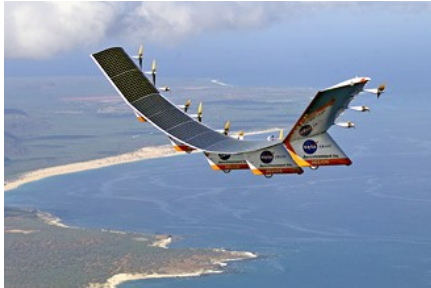
Fig. 1.5: Helios aircraft (NASA) powered by a regenerative fuel cell system and photovoltaic modules. (Source: NASA Archive Website)
