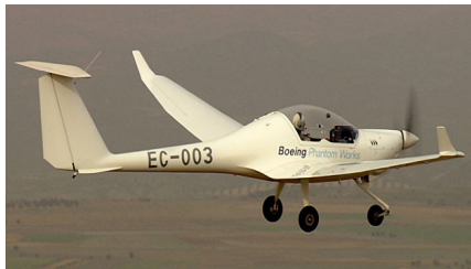
Fig. 1.6: Boeing's fuel cell aircraft, one of the first examples of manned fuel cell aircraft.
