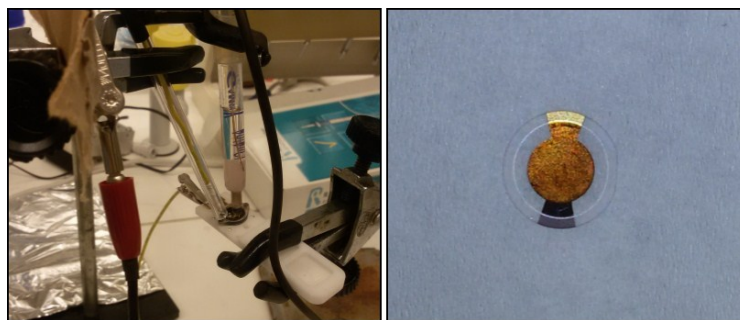
Figure 4.3: Experimental set-up for the electrochemical synthesis (on the left); and a gold coated quartz resonator with the MIP thin film on the top after the electropolymerization (on the right).
