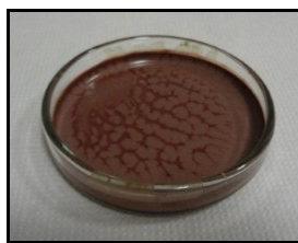
Figure 3.28: PMMA/TiO 2 film with 15 wt% NPs impregnated with TCPP in the Petri dish.
