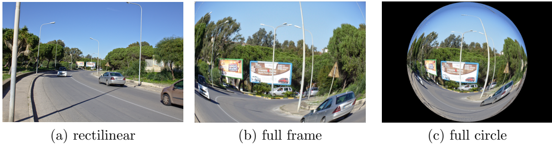
Figure A.6: Examples of perspective (a), full frame (b) and full circle (c) images. The two fisheye images are obtained by artificially adding different amounts of radial distortion to the rectilinear image (a).
