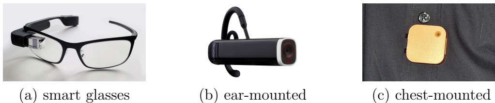
Figure 2.2: Three devices involving different wearing modalities: (a) smart glasses, (b) ear-mounted wearable camera, (c) chest-mounted wearable camera
