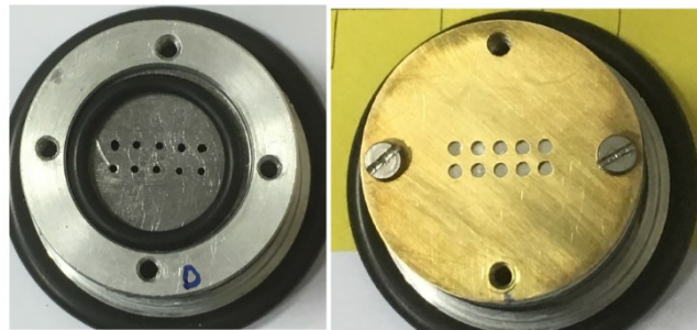
Fig. 3.3.2 – An eight-pinhole array on the left and Al-made attenuators on the right.
