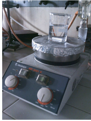
Fig. 4.2. Hot plate/stirrer used for chemical roughening and polymerization.
