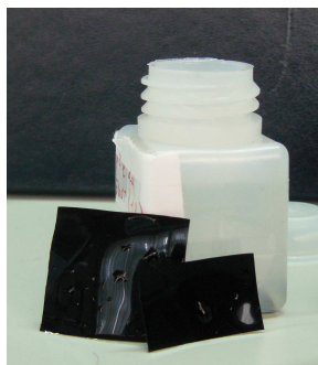
Fig. 4.3. Membrane of IP 2 C realized through electrodes polymerization.
