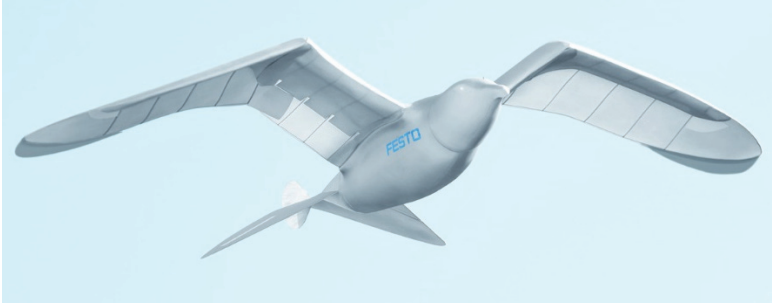
Figure 8 - Flapping wings, bird-like airframe
