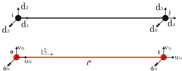
Figure 4.15 Relationship between local and global degrees of freedom in the external edges.
