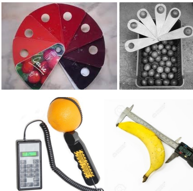
Figure 1.1. Sizer used commonly in field (above left and right, respectively) and electronic digital slide gauge with 0.01 mm accuracy (below left and right, respectively)
