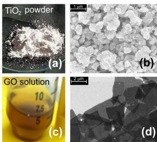
Figs. 33. A) Picture of  $\text{TiO}_2$  powder; B) SEM image of aggregates of  $\text{TiO}_2$  nanoparticles; C) Picture of GO dispersed in water solution; D) SEM image of GO flakes (from Pecoraro *et al.*, 2017).
