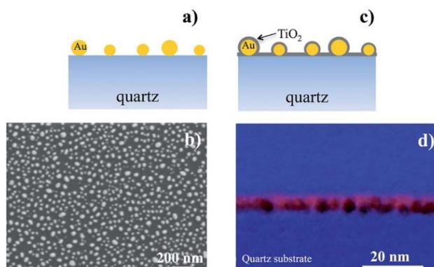
Figs. 22. A) Scheme of the AuNPs on the quartz substrate just after the thermal process and B) the relative plan-view SEM image; C) Scheme of the sample after the  $\text{TiO}_2$  deposition by ALD and D) the relative EF-TEM image in false colors ( $\text{TiO}_2$  is denoted in magenta and Au nanoparticles in black) (from Scuderi *et al.*, 2014).
