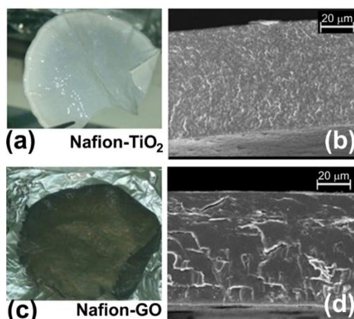
Figs. 34. A) Picture of a Nafion- $\text{TiO}_2$  membrane; B) SEM image of a cross section of the membrane; C) Picture of a Nafion-GO membrane; D) The same membrane observed by SEM in cross section (from Pecoraro *et al.*, 2017).
