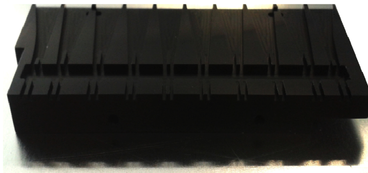
Figure 4.3 - Picture of a cookie that guide the WLS fibers to the SiPMs.
