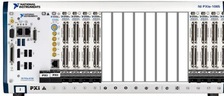
Figure 4.20 - A picture of the PXIe-1065, 18-Slot 3U PXIe/PXI Chassis, including the real-time module, the GPS timing module and the eight PXI-7813 digital sampling board.
