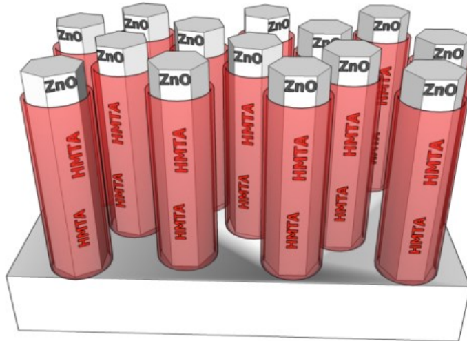
Figure 2.25: Illustration of the shaping effect of HMTA in ZnO NRs grown by CBD.
