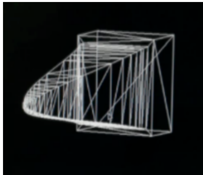
Figure 4.9: Single pin of the ridge filter geometry imported in Geant4
