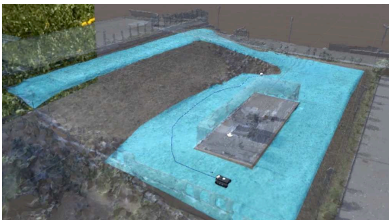
Figure 4.12 The traversable area represented as a cyan layer overlaid onto the environment model reconstruction
