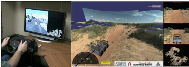
Figure 4.10 The operator control station and a view of the interface by Kelly et al. (image from [41] ©2011, SAGE Publications)
