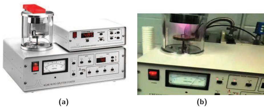
Fig. 6.6. Golden covering realization: (a) manual sputter coater machine; (b) a picture of machine used.
