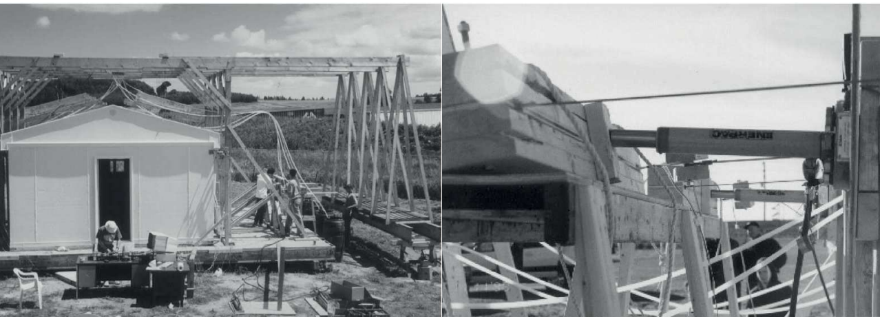
Figure 77 / The Department of Civil and Environmental Engineering of the University of Western Ontario in London, Canada, carried out an experimentation survey on a full-scale prototype of a shelter of DuraKit Shelters Inc., verifying its resistance even under the heavy loading conditions of tropical winds - ◀ Overall view of test facility, 2003 - © Michael J. D'Costa, F. Michael Bartlett - Journal of Wind Engineering and Industrial Aerodynamics 91 - Elsevier
