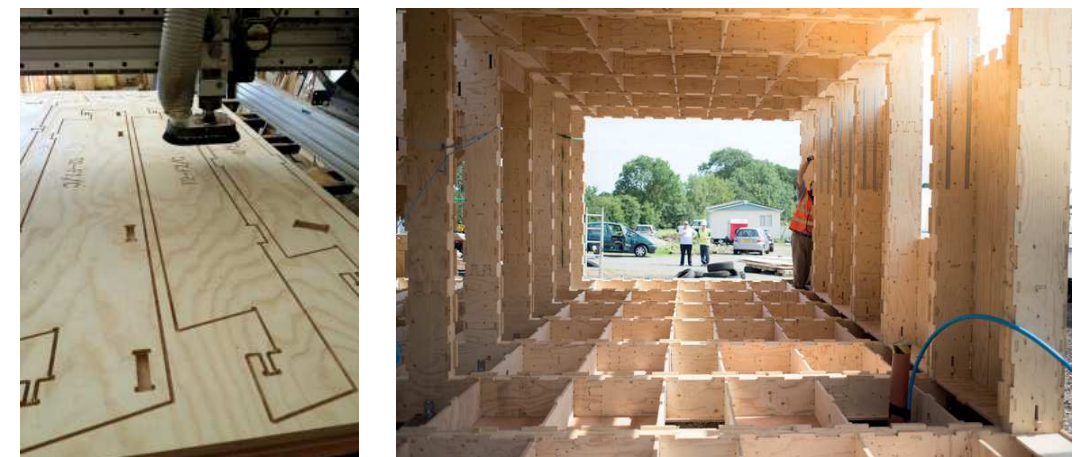
Figure 37 / ▼ Wikihouse CNC cutting and prototyping - © www.architecture00.net
