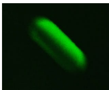
Figure 32. Image of the non homogeneous fluorescein distribution in a droplet.
