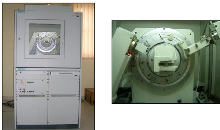
**Fig. 5.1** Diffrattometro modello SIEMENS D5000.
