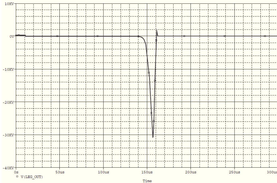
Fig. 3.9: Leg output voltage, measured respect to the midpoint of the DC bus voltage, for the isolation topologies proposed by Ribeiro et al and Bolognani et al.
