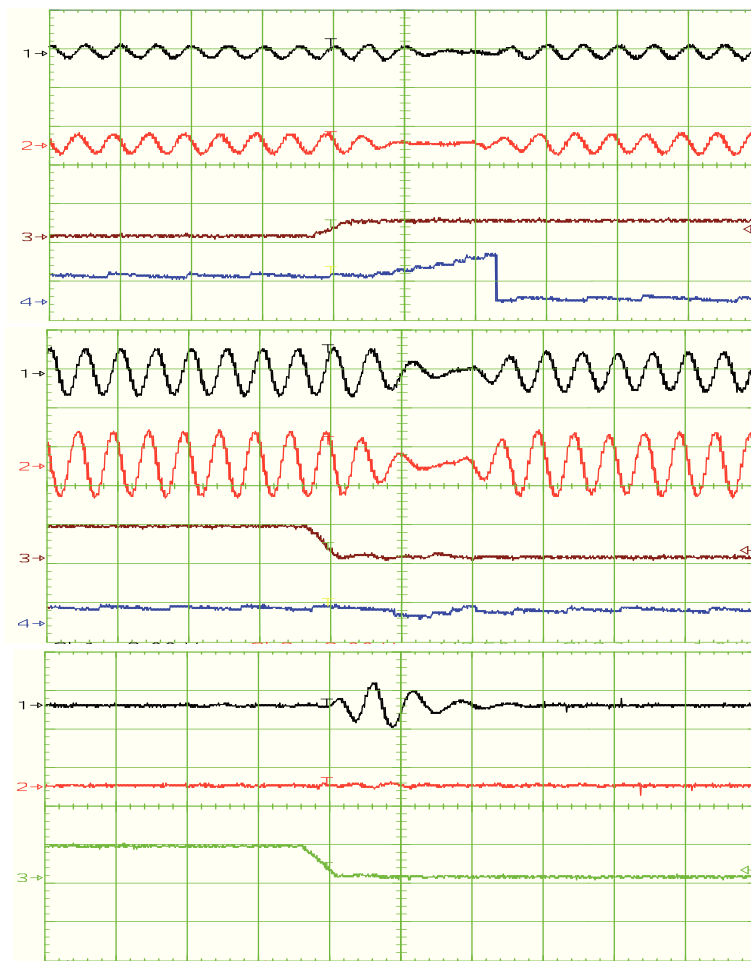
Fig. 7.2: Effects of transient components of the stator current at locked rotor during torque steps. CH1)-CH2) band-pass filters outputs [0.2 A/div] CH3) C_e [9 Nm/div.], CH4) \theta_{re}^{est} [ \pi rad/div.] Time [2.5 ms/div.]
