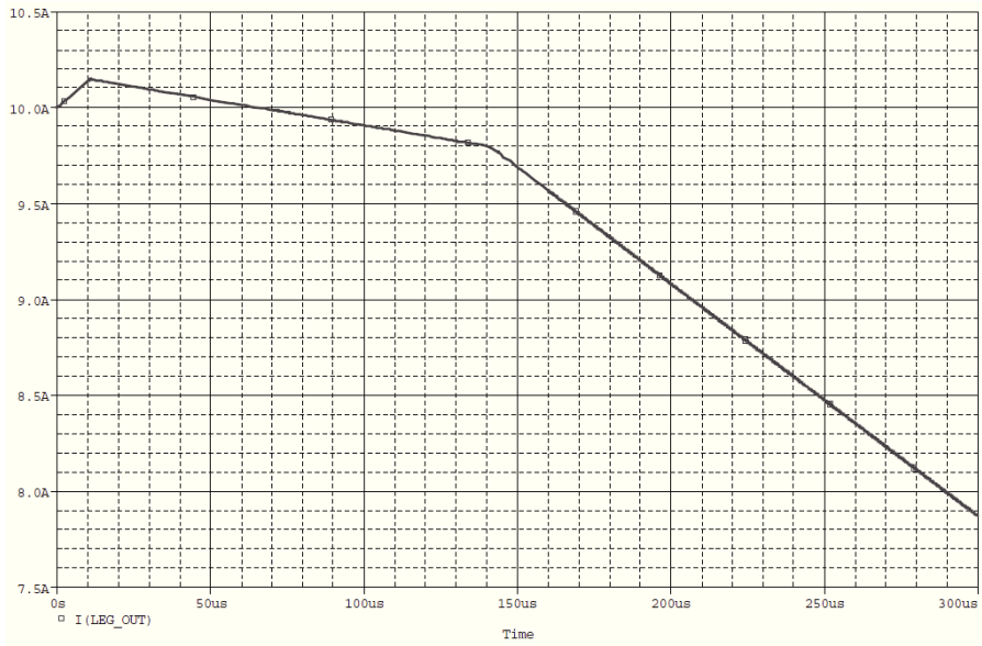
Fig. 3.11: Leg output current for the proposed isolation topology.
