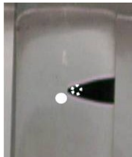
Figure 3-23 a) real view of the device; b) zoom of the ferrofluid spike; the IR emitter diode is represented by a dotted circle while the photodiode is represented by a filled white circle.
