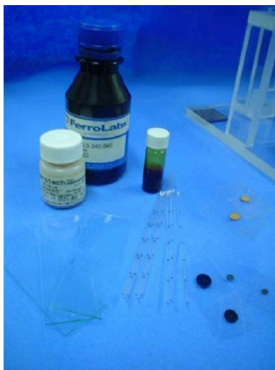
Figure 4.2.4 - Overview of some of the magnetic tracers used in the experimental tests.
