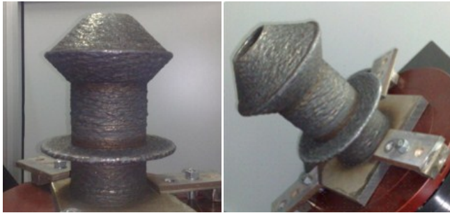
Figure 3.12 Stainless steel 316 structure deposited using 2 axis rotating table
