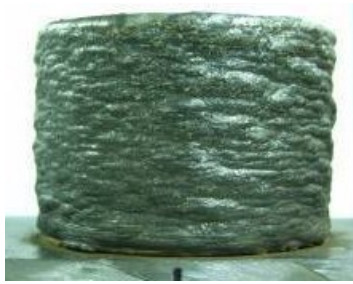
Figure 3.8 A cylinder deposited with stainless steel
