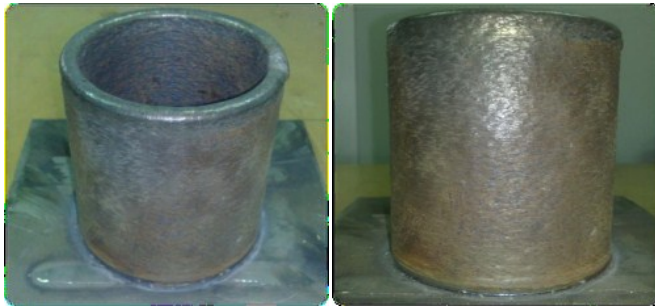
Figure 3.13 Titanium cylinder deposition
