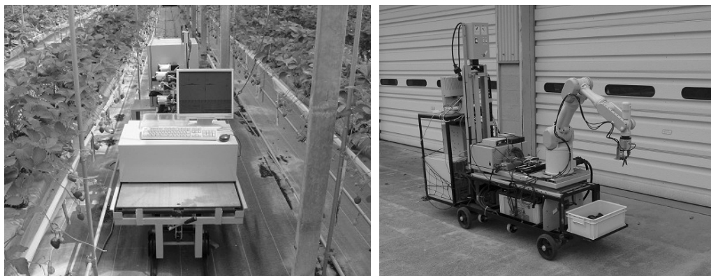
Figure 9 - Strawberry and eggplant harvesting robot
