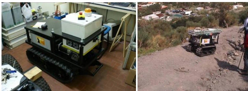
Figure 33 - The tracked U-Go Robot in the lab and during a teleoperated outdoor test.
