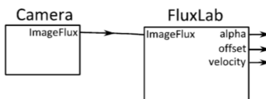
Figure 47 - Block diagram of the implemented software.
