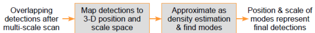
Figure 88 - An overview of the steps of the non-maximum suppression algorithm. The detection window is scanned across the image at all positions and scales, and non-maximum suppression is run on the output pyramid to detect object instances.
