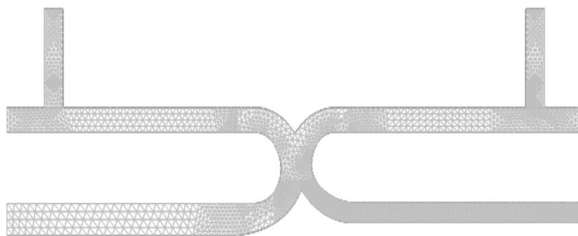
Figure. 2.28. Refined Meshing of the Geometry
