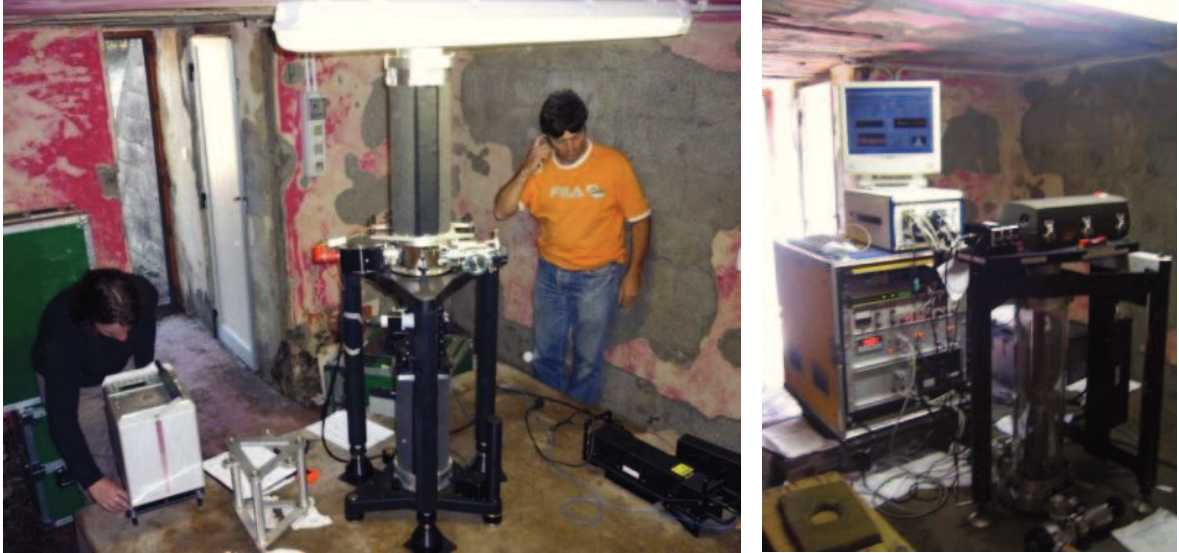
Figure 2.3 – Gravity station at Serra La Nave (Mt Etna): on the left the FG5#238 and on the right the IMGC-02.
