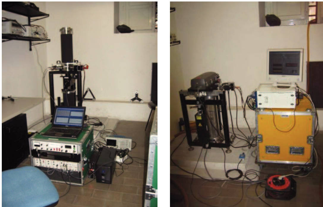
Figure 2.1 – Gravity laboratory at Catania (INGV): on the left the FG5#238 and on the right the IMG-02.
