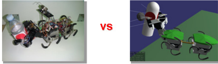
Fig. 9.1. Comparison of real and simulated TriBot I version. In these screenshots it is possible appreciate the high fidelity of the simulated reproduction.
