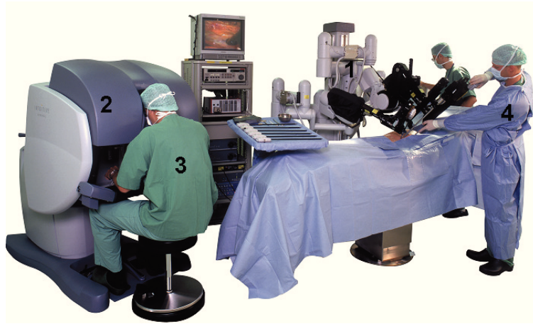
Figure 9.1: The surgical robot “DaVinci”. It consists of four entities: 1) a plenty of surgical instruments and 2) the console to handle them by the surgeon (3). His assistant (4) works next to the robotic arms and the patient.
