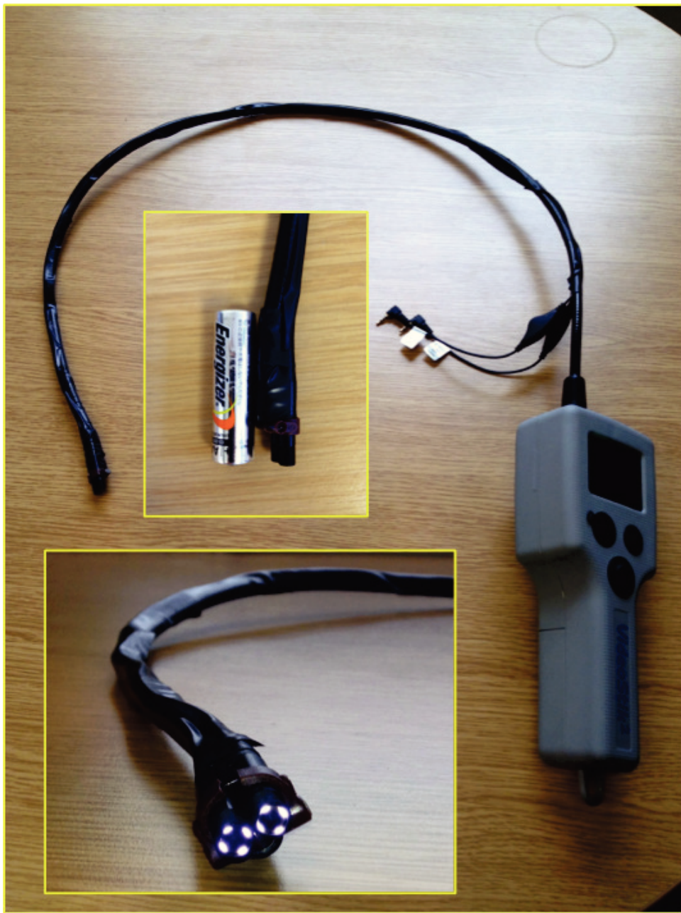
Figure 10.11: The prototype of flexible stereo bronchoscope. The cameras are placed at the end of a probe whose tip can be articulated by the user in two directions up to 180^\circ . The best configuration has been obtained with the cameras perfectly adjacent with parallel optical axes.
