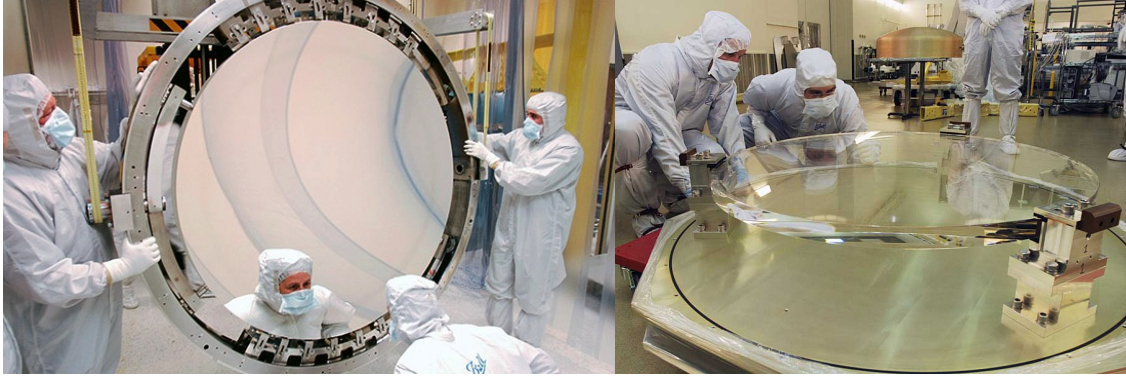
Figure 3.3: Pictures of the 1.4 m mirror (left) and of the 0.95 m Schmidt corrector (right).
