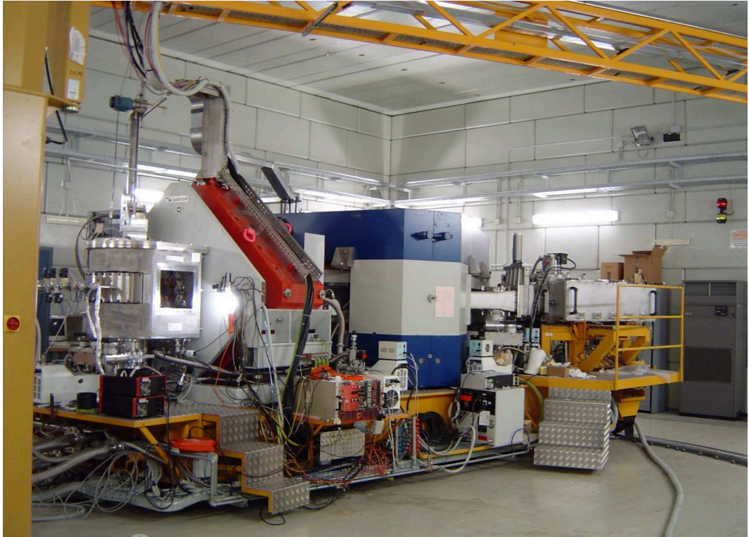
Fig. 5.3. General view of the MAGNEX spectrometer. From the left to the right, the scattering chamber, the quadrupole (red) and the dipole (blue) magnets and the Focal Plane Detector are visible.
