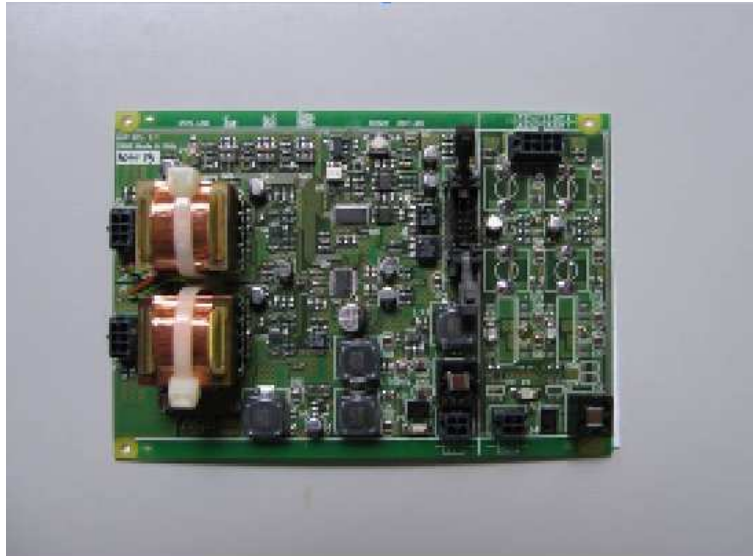
Figure 5.8: Picture of the AcouBoard. The AcouBoard distributes the power to the preamplifiers and performs the digitization of the acoustic signal at a frequency of 192 kHz with a resolution of 24 bit.
