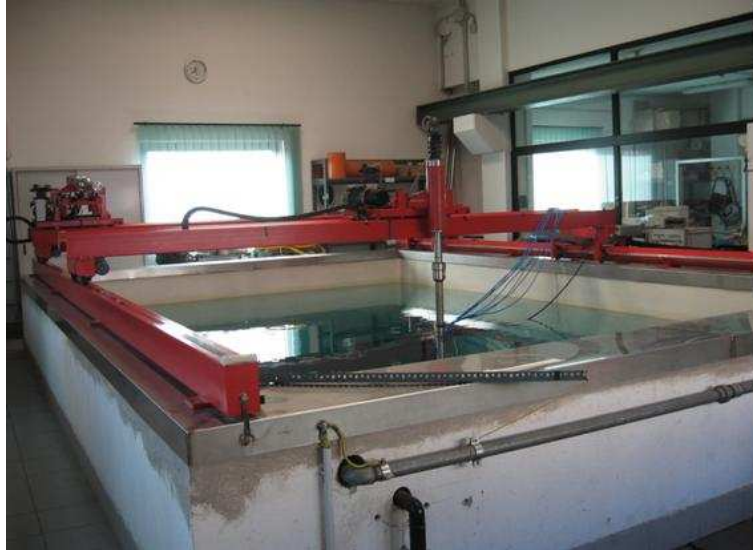
Figure 6.5: Picture of the CNR-IDASC waterpool, used for the tests in water of the SMO hydrophones.
