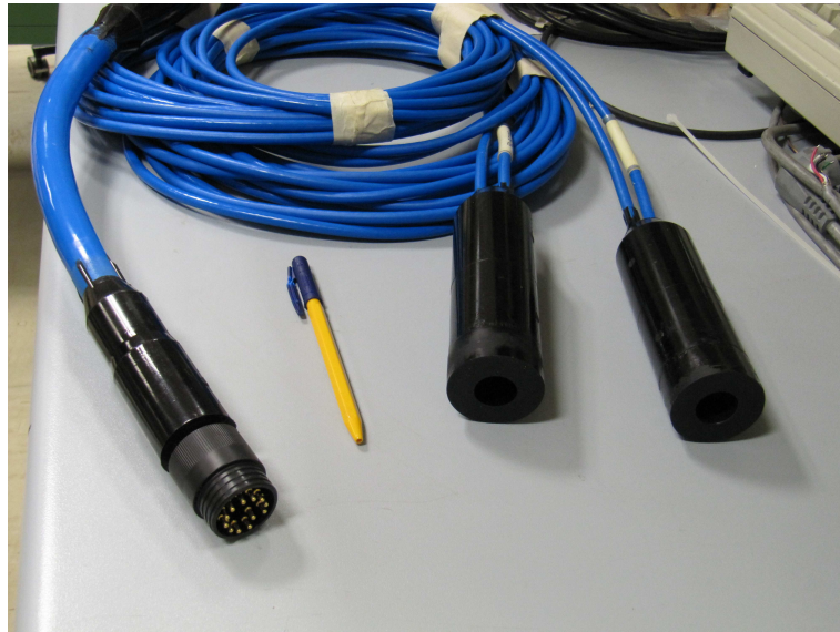
Figure 5.4: Free flooded rings hydrophones Sensor Technology Ltd SX-30 + SMID AM-401(V)1 preamplifiers, moulded in a deep-sea cable 7.5 m long.
