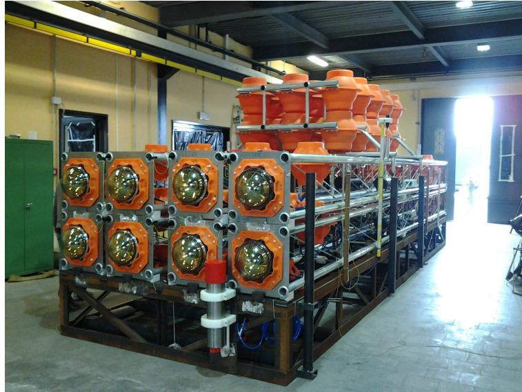
Figure 4.4: The NEMO-SMO tower in compact configuration during the integration phase.
