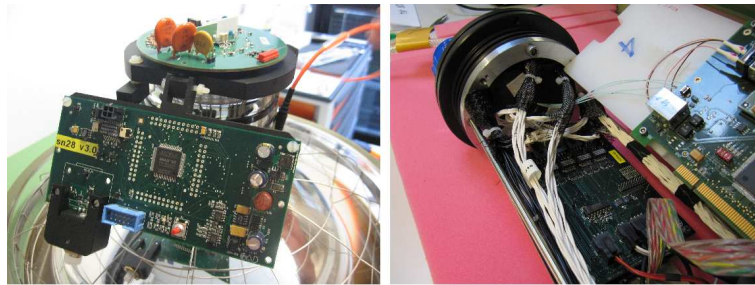
Figure 4.19: Left: TimCal Board installed in the OM. Right: Picture of the TimCtrl board into the FCM
