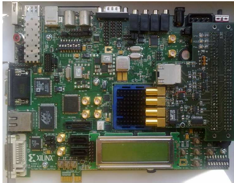
Figure 4.14: Ethernet Floor Control Module Board based on Virtex 5 board. The board receives and parses the underwater data stream, that can be accessed by the on-shore data acquisition system through Gigabit Ethernet connection.
