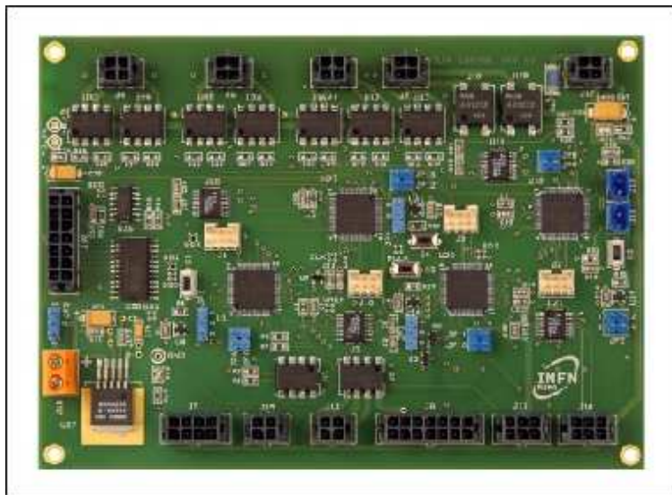
Figure 4.25: Picture of the Slow Control Interface (SCI). The SCI is interfaced with environmental instrumentation using serial ports (RS-232).
