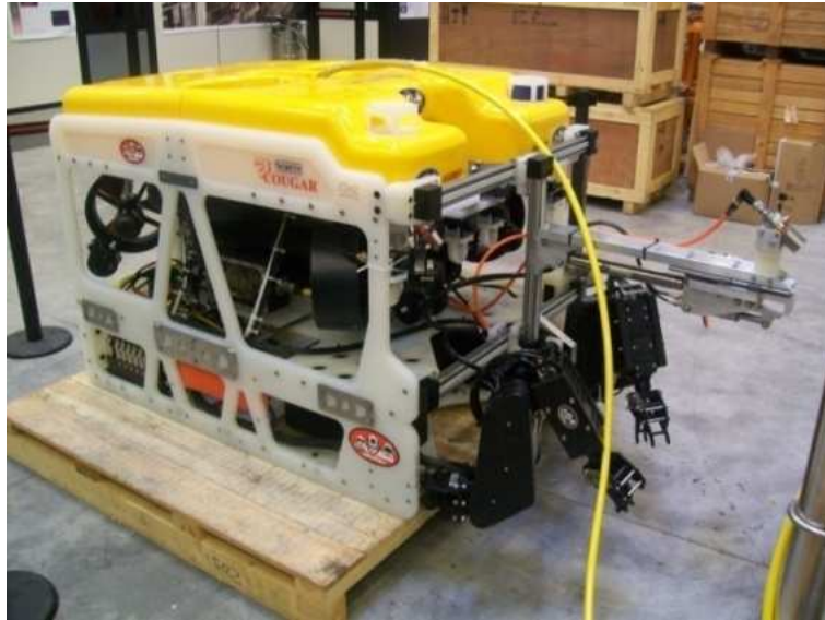
Figure 4.3: Picture of the The PEGASO ROV. It will be employed in the installation of NEMO-SMO detector at a depth of 3500 m.
