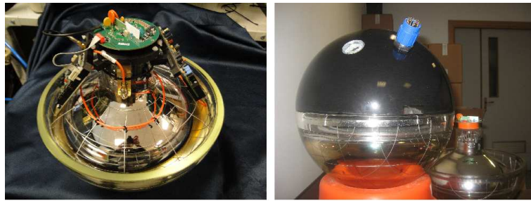
Figure 4.10: Left: Semi-sphere of optical module holding the photomultiplier and the Front-End Module board. Right: Optical module fully integrated with connector and pressure meter.
