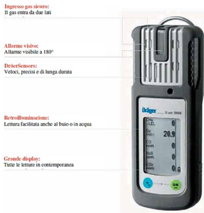
Fig. 4 - Portable instrument for the measurement of ammonia concentration (Dräger, Germany)
