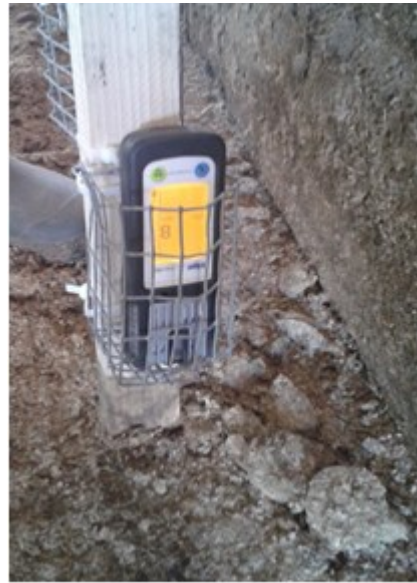
Fig. 23 - Ammonia concentration measurement with the portable instruments placed in the wooden facility, after the treatment.
