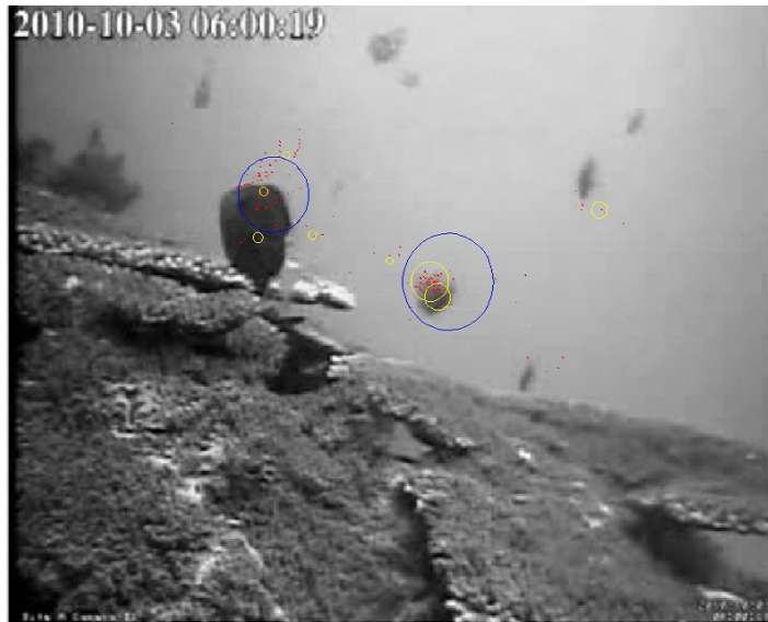
Figure 3.2 - Clustering applied on the acquired data: Red dots are the locations clicked by the users. Yellow circles represent the result of the first clustering iteration, while the blue circles are the final result of the clustering method. The radius of each circle is equal to the sum of the quality scores of the users that made an annotation that belongs to that cluster, given by equation (3).
