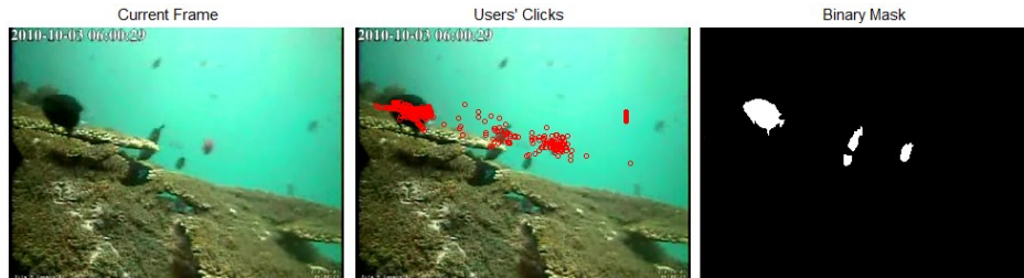
Figure 3.12 – Final segmentation results. On the left , the source image as presented to the user during the game session. In the center image , the users clicks obtained for the current frame. On the right image , the binary mask with the segmented objects.
