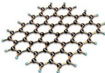
Figure 2.4 – A graphene sheet, where the carbon atoms are arranged in a honeycomb lattice.
